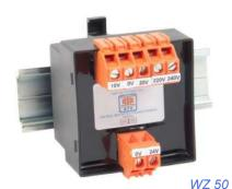
A new and unique range of DIN rail mountable, fully encapsulated, custom-built single-phase transformers meeting Class II double insulated (with no provision for earth). All transformers are enclosed in a black, high quality, flame retardant housing to UL 94. Rating options are from 25VA to 50VA with IP20 touch-proof terminals. The ambient temperature range is between  $-10^{\circ}$ C to +35 °C with the maximum voltage being 500V. The frequency for the models within this range is 50 / 60 Hz.
