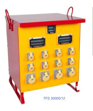
The TFS range of portable site transformers with 400~420V 3ph delta connected input are suitable for a number of applications. There are five models from 10kVA (12.5kVA tool rated) to 30kVA (35kVA tool rated). Units are fitted with either 6, 9, or 12 sockets with all inputs and outputs being MCB protected with the MCBs mounted behind an IP65 rated, high impact, hinged window. The steel enclosure is to Class 1 construction and is phosphor pre-treated and epoxy powder coated red and yellow.
