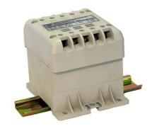
A new and unique range of custom built single phase transformers meeting Class II (with no provision for earth). All transformers are enclosed in a grey, high quality, flame retardant moulded housing to UL94VO with terminals protected to IP20.
