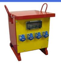
A range of stock (MV) single phase or 2 wire (2ph) enclosed transformers for various applications. These are cased in a variety of enclosures with 110V centre tap to Earth outputs or 240V outputs. Output sockets to BS 4343 can be fitted. Either fuse or MCB protection can be fitted either internally inside the enclosure or on the front in an IP65 rated accessible cover. A basic example is shown above. Other types are available.
